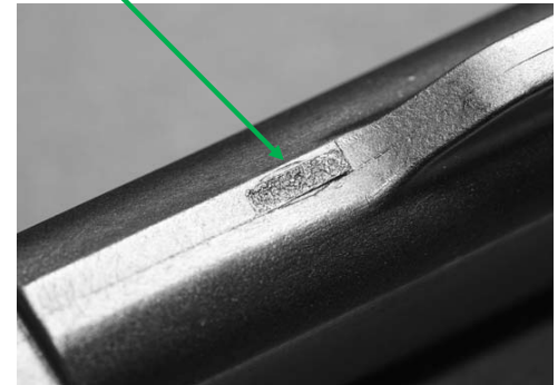
Tab gate blemish along parting line on a MIM component.
