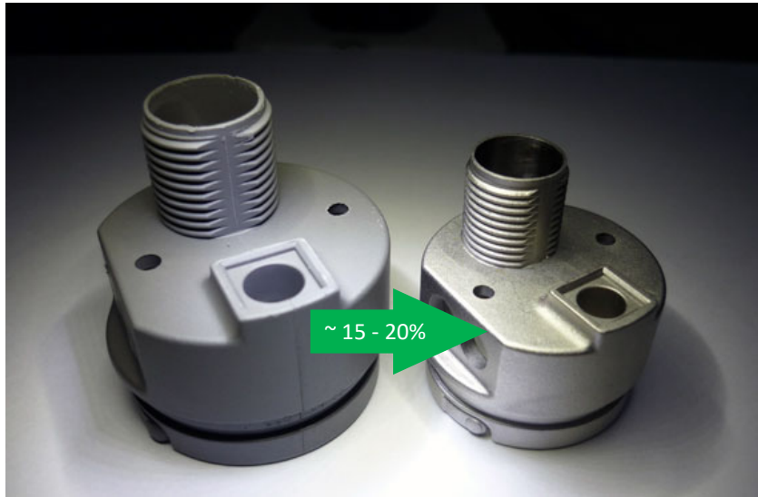
Metal Injection Molded housing cover made from 316L stainless steel (sensor casing). Before and after sintering. (source PIM International Vol.4 No.1, March 2010)
